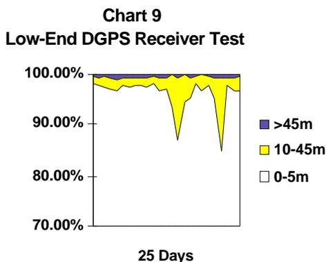
The 2-sigma value and the 95% CEP (Circular Error Percentage) values were close (ranging from 3.67 m to 11.00 m) and the overall mean was 2.03 m. This test also showed that a maximum distance error ranging between 150 m and 200 m was observed on most days, suggesting
