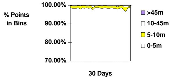
Although the daytime signal strength at Canberra (Chart 3) was only 30 dB $\mu$ V/m, the accuracy was found to be better than 5 m 95% of the time with a recorded SNR of 10 dB. This is significant as the results show that in areas where there is low man-made noise or atmospheric noise, the DGPS signal can be received with good accuracy much farther than that specified by AMSA. (AMSA's specification of 95% availability is defined as distance where daytime signal strength is 42 dB $\mu$ V/m.)
