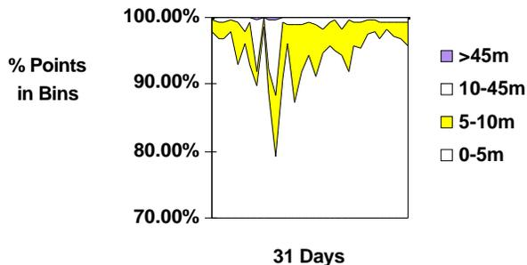
From the results of Chart 7 it is obvious that the accuracy was significantly better in the quieter location. Only three observation days had an accuracy worse than 10 m 95% of the time due to a high level of thunderstorm activity. On the worst day about 89% of the position errors were less than 10 m. Close examination showed that for these three days the actual radial error bin for 95% of time was the 10-15 m bin. The daytime signal strength received at the Cairns suburb was 51 dB $\mu$ V/m.
