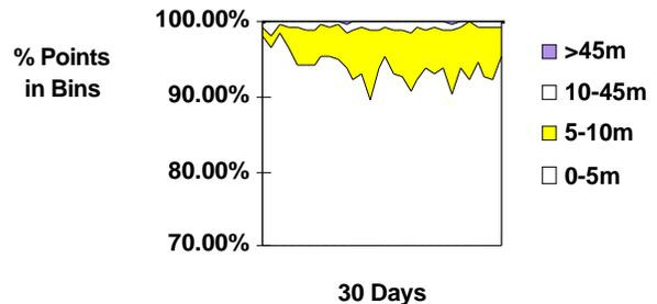
At Rosslyn Bay the received daytime signal strength was 42 dB $\mu$ V/m, and was, therefore, on the boundary of AMSA's assumed coverage. From Chart 5 it can be seen that for 95% of the time, 9 of the 30 days had position errors in the 0-5 m bin while the remainder were in the 5-10 m bin. Hence, it can be assumed that the Mackay service extends beyond 150 NM for an over land path.
