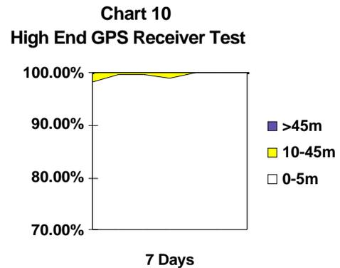
The 2-sigma value and the 95% CEP values were again close and more accurate than for the first test (ranging from 0.79 m to 3.15 m). The overall mean was 0.71 m.
